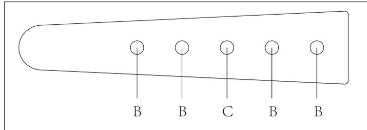
Connect sofa legs(D) by tightening Screws(C) through the third hole on sofa leg to the position hole on sofa. Using the self-tapping screws(B) for other hole on sofa legs.
